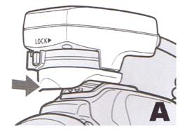
Slide the lock lever to the right until the lock lever clicks into place. The cord will be locked onto your camera hot shoe.
