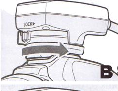
■ To detach the camera connector, press the lock-release button and slide the lock lever to the left. Slide the camera connector out of your cameras hot shoe to remove.
